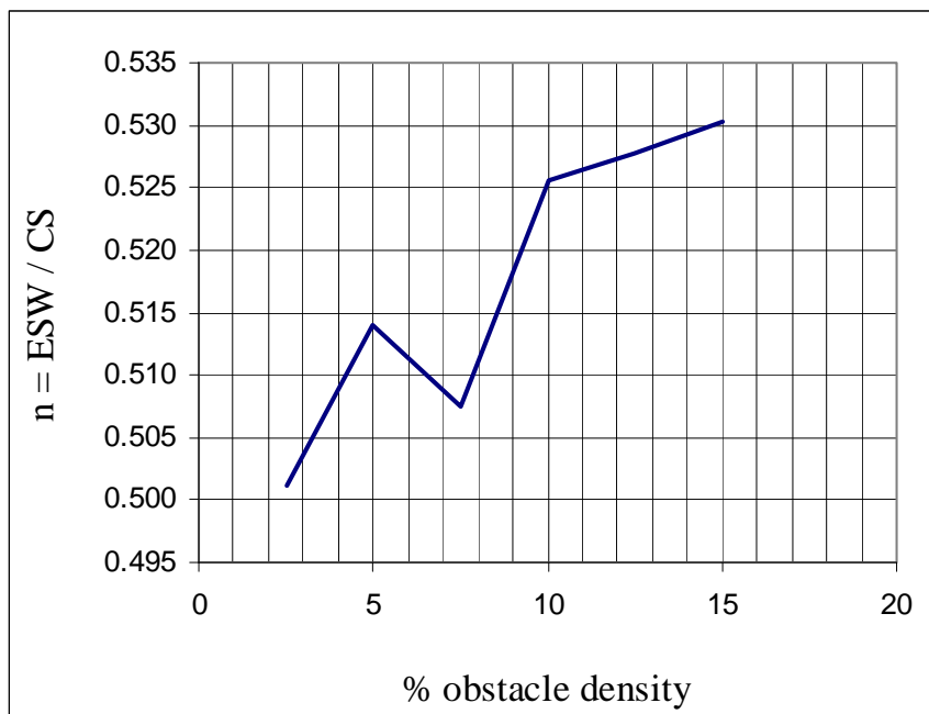
Fig. 7: graph of n against percentage obstacle density for the standard set of experimental obstacle densities
